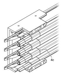
Fit the multipole bar (a) onto the connectors (b) and slide it until there is no gap (c) with the joint body.
