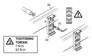
Place the groove of the conductor (a) on the notch of the support (b) and push the conductor (c) towards the support (d).
