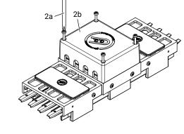
Remove the locking bar (a) and make the wiring fastening each pole into the corresponding block (b) with an Allen key.
