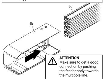
Fasten the lateral screws to fix the feeder body to the multipole line.
