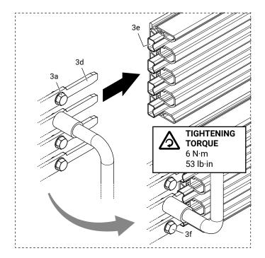
Loosen the M5 bolt (a) and slide the feeder body (b) on the multipole line (c) in order to insert the pins (d) into the copper conductors (e) and then tighten the bolts (f).
