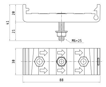
The unit consists of 1 support clip (a), 1 allen screw with nut (b) and 2 fixing screws (c).
