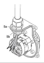
Fix the cable gland (a) and then tighten the lock nut (b).
