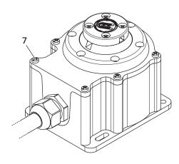
Refit the cover on the base with the 6 screws.
