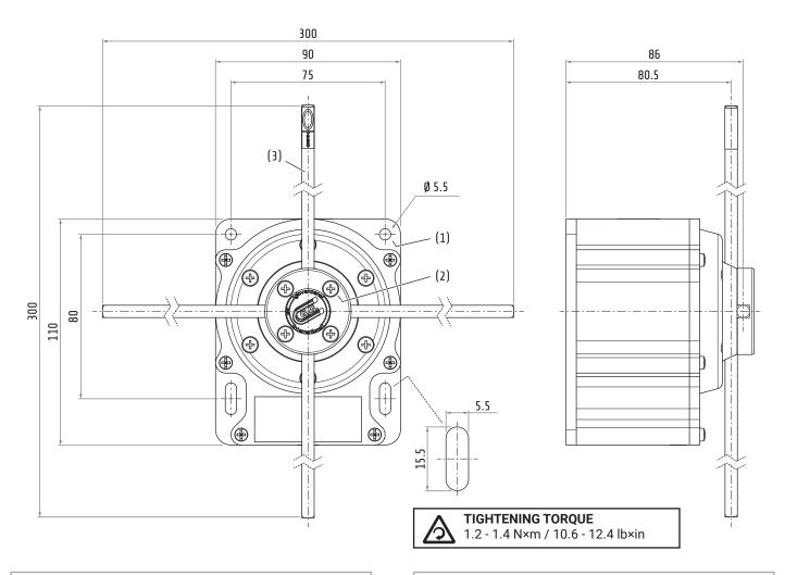
Fix the limit switch with 4 suitable screws (1) (not supplied) into the service position, considering the drilling pattern and the overall dimensions shown in the picture.
