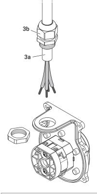
Insert a suitable cable (a) into the cable gland (b).
