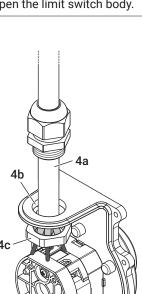
Insert the cable (a) in the limit switch cover (b) passing it also through the lock nut (c).
