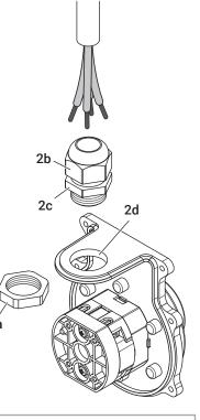
2 Loosen the lock nut (a) of a cable gland (a-b-c) matching the Ø 22.5 mm hole (d) of the limit switch.
