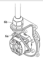
Wire (a) the cam switch according to the diagram in paragraph "Cam switch operation" p.8. After wiring, tighten the sealing nut (b).
