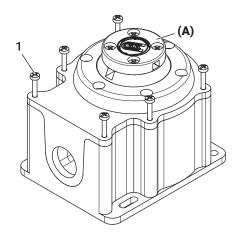
Unscrew the 6 screws and open the limit switch body.
